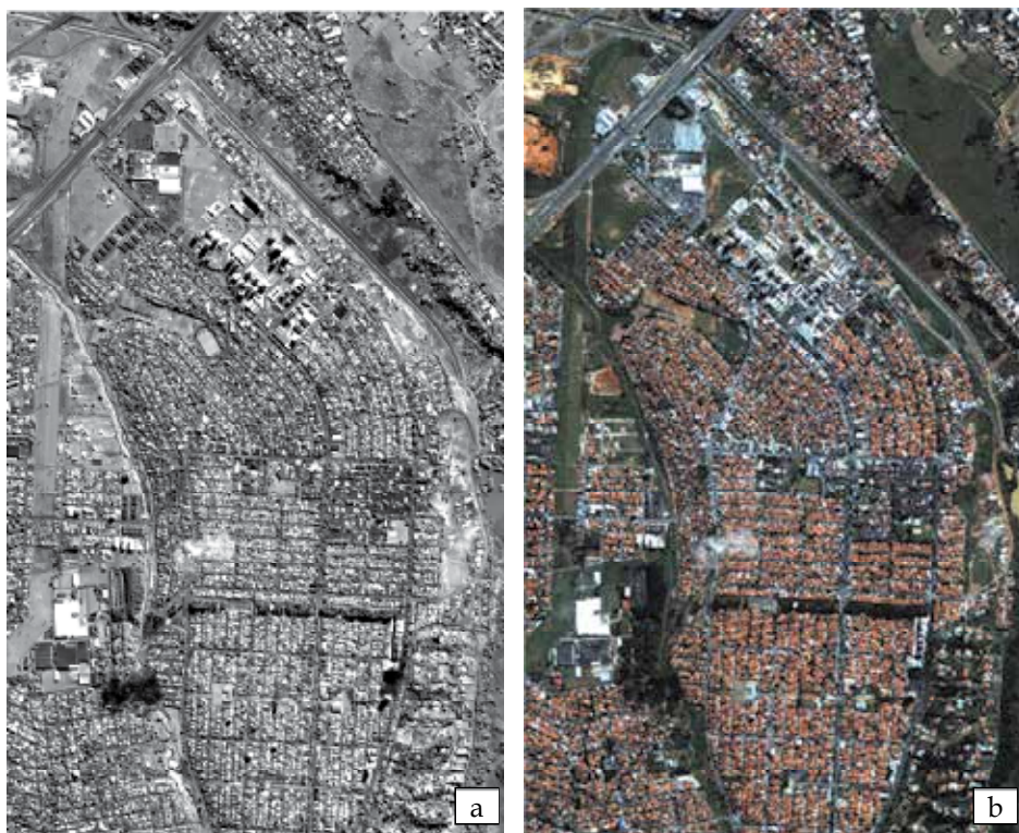
Fig. 12. Quickbird satellite scene acquired on 05/17/2004: (a) panchromatic image (0.6 m), and (b) multispectral image (2.4 m), (band 3 in red, band 2 in green and band 1 in blue).
