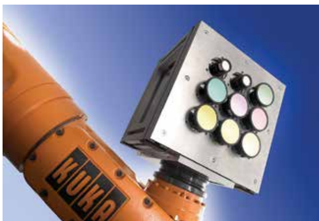
Fig. 1. Camera array used for the acquisition of combined image series. The cameras are equipped with spectral filters.
