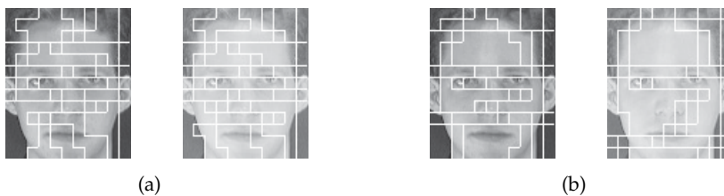
Fig. 35. Viterbi segmentation of face images under different illumination conditions using edge-based feature vectors (a) and DCT-based feature vectors (b); each block corresponds to each state of pseudo-2D HMM.
