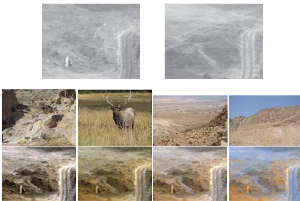
Fig. 4. Fusion results of applying the P-AOCT method with different target images to the Dune images of a nighttime scene representing a person walking over a dune area covered with semi-shrubs and sandy paths. Top left: the input 3-5 \mu\text{m} midwave infrared image. Top right: the input visible image. Middle: four different target images. Bottom: the corresponding fusion results corresponding to each target image. (The two left target images courtesy of www.pics4learning.com , and the two right target images courtesy of www.bigfoto.com .)
