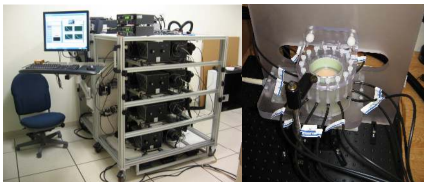
Fig. 3. The experimental spectrometer-based system depicted at left couples directly into the MR via 13 meter fiber optic bundles. Sixteen spectrometers are computer controlled for rapid image acquisition (left photograph). An animal interface (right photograph) is composed of a rodent MR coil custom built by Philips Research Hamburg to accommodate the optical fiber array for simultaneous MR and NIR fluorescence imaging.
