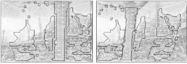
Figure 7. The result of the joint view triangulation: the black edges are the boundary edges of the matched regions and the white edges are Delaunay edges which are not matched.
