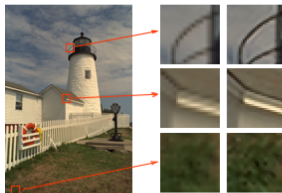
Figure 4: Comparison of visual quality for bilinear interpolation (left) and the proposed super-resolution algorithm (right).
