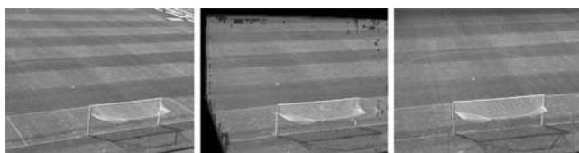
Fig. 9 Rendering an intermediate novel view from 2 cameras 13 m apart. Note that the reconstructed novel view preserves both high (pitch lines) and low (grass stripes) frequencies
