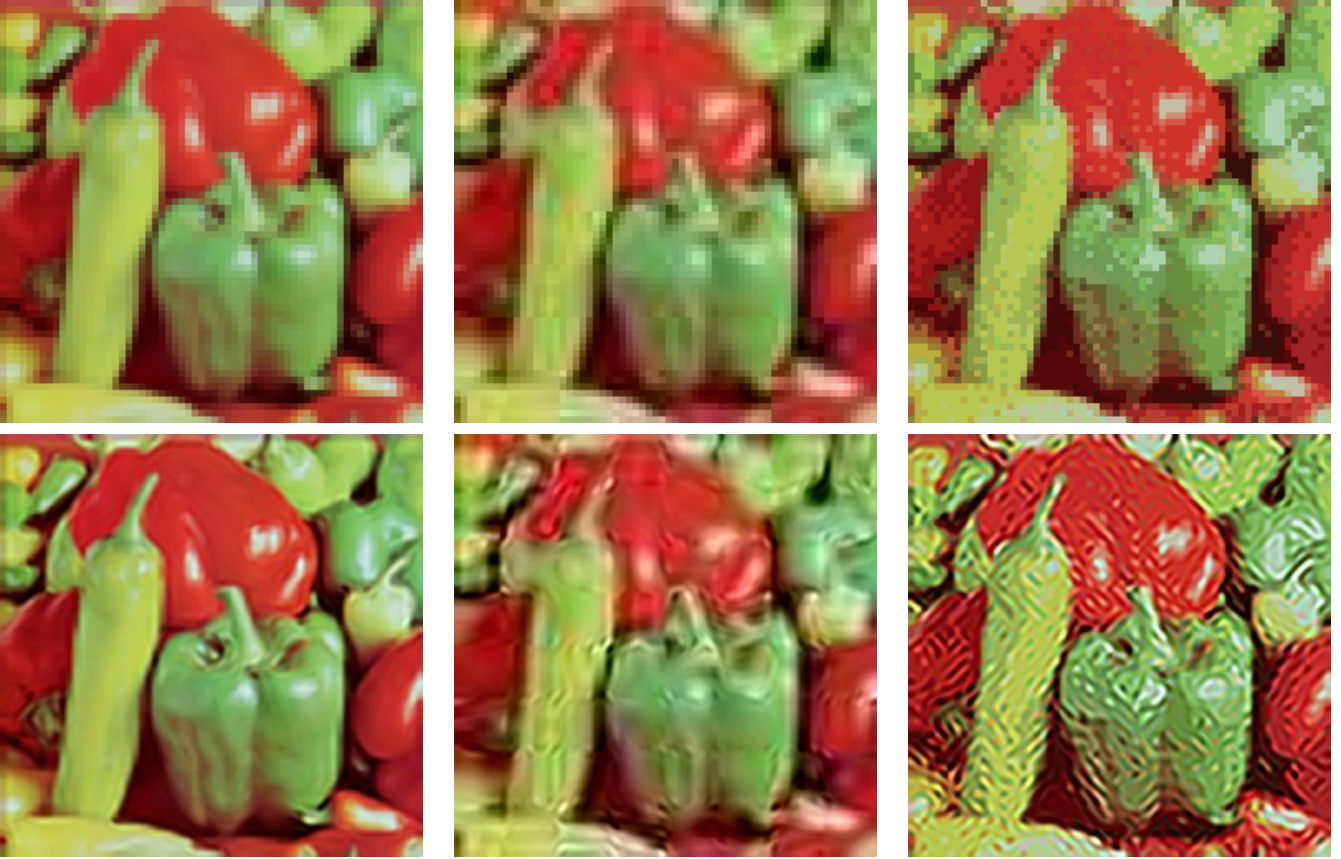
Figure 8: Interpolation results on noisy images. The top row shows the input images, from left to right: clean input, JPEG compressed and quantized colors. The bottom row shows their interpolations, from left to right: PSNR 26.48, MSSIM 0.8196; PSNR 20.38, MSSIM 0.5244; PSNR 18.30, MSSIM 0.3393.
