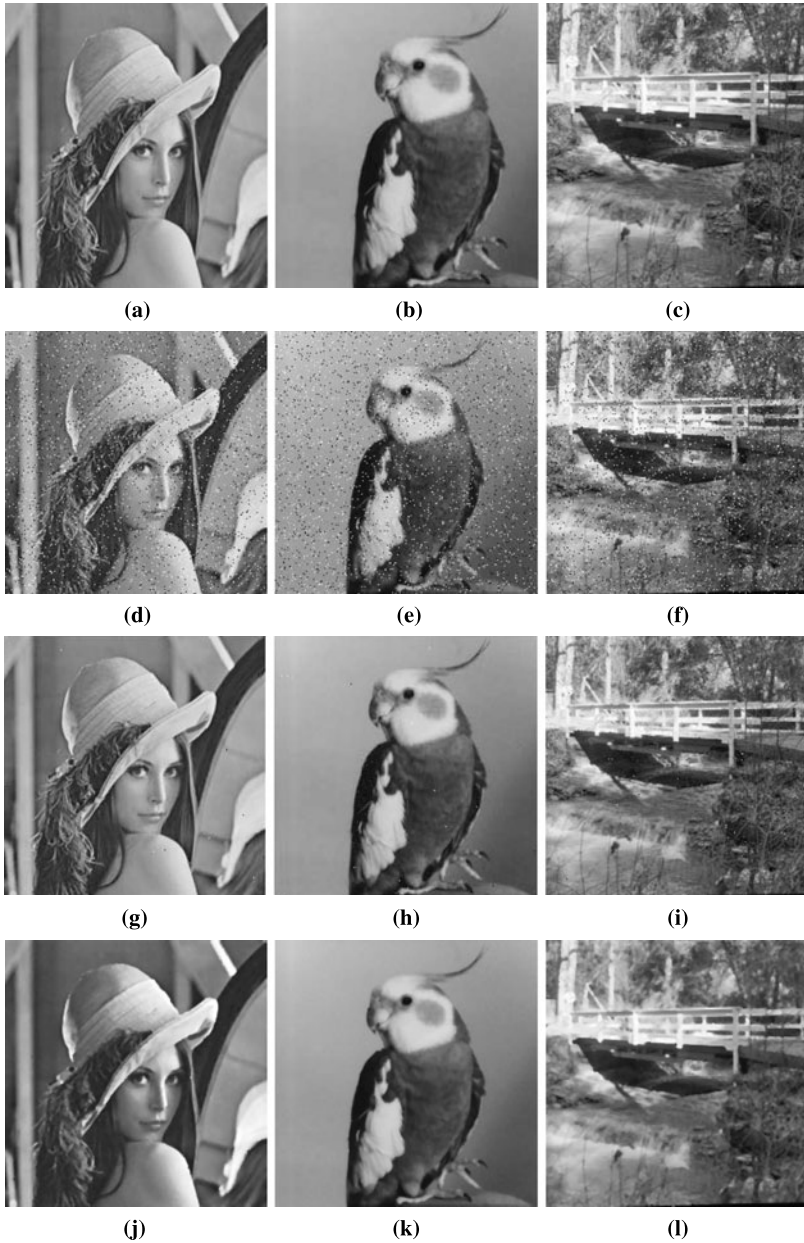
Fig. 6.6 Original images (a, b, c), images with salt-and-pepper noise (d, e, f), images filtered using an evolved filter (g, h, i) and images filtered using a median filter (j, k, l). The evolved filter was trained via the Lena image (a, d).
