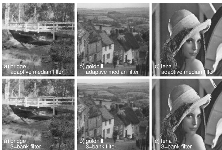
Fig. 6.9 Comparison of images filtered using an adaptive median filter with a kernel size of up to 7 \times 7 (a, b, c) and using a three-bank filter (d, e, f).
