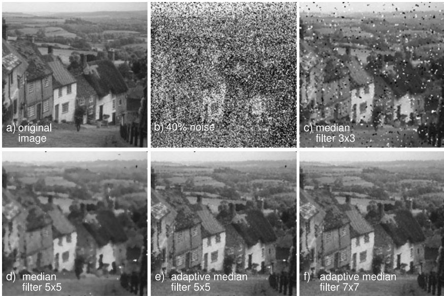
Fig. 6.3 Images obtained by using conventional filters. (a) Original image. (b) Noisy image with 40% salt-and-pepper noise (peak signal-to-noise ratio (PSNR) 9.364 dB). (c) Filtered by median filter with a kernel size 3 \times 3 (PSNR 18.293 dB). (d) Filtered by median filter with a kernel size 5 \times 5 (PSNR 24.102 dB). (e) Filtered by adaptive median filter with a kernel size of up to 5 \times 5 (PSNR 26.906 dB). (f) Filtered by adaptive median filter with a kernel size up to 7 \times 7 (PSNR 27.315 dB).
