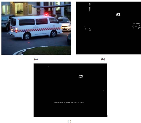
Fig. 4 : a) Image of a vehicle during daytime, (b) Detection of all lights, (c) Emergency vehicle detected
