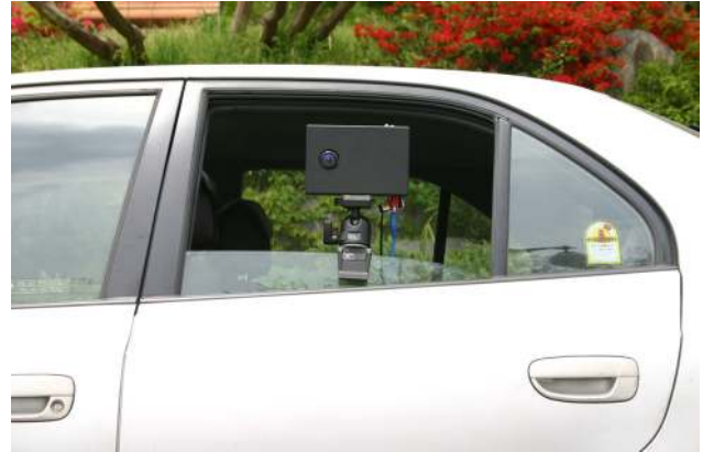
FIG. 14. The panoramic camera mounted on a side-window of a passenger car.
