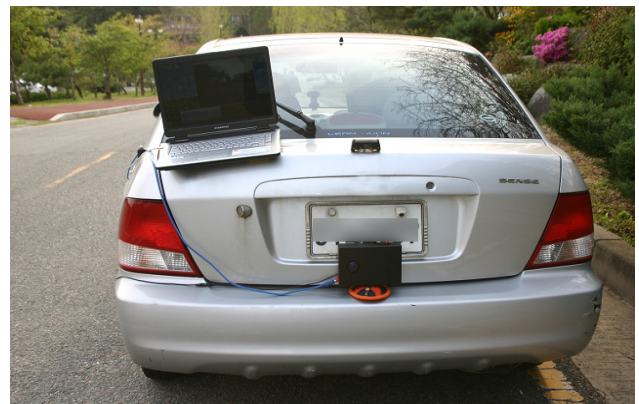
FIG. 16. The panoramic camera installed near the rear bumper of a passenger car.
