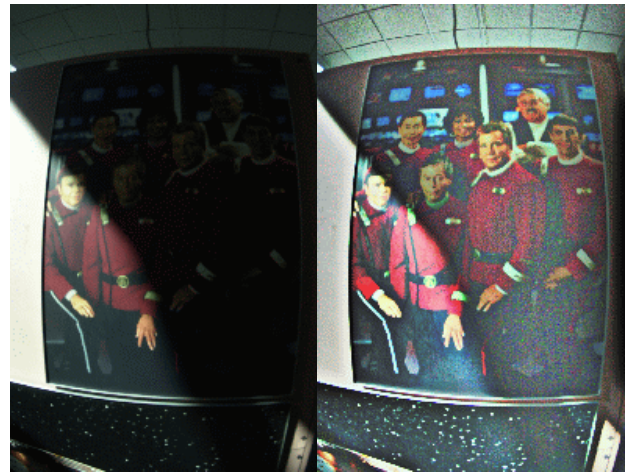
Figure 11: A successful example of adapted Retinex processing on a traditional brightening task
