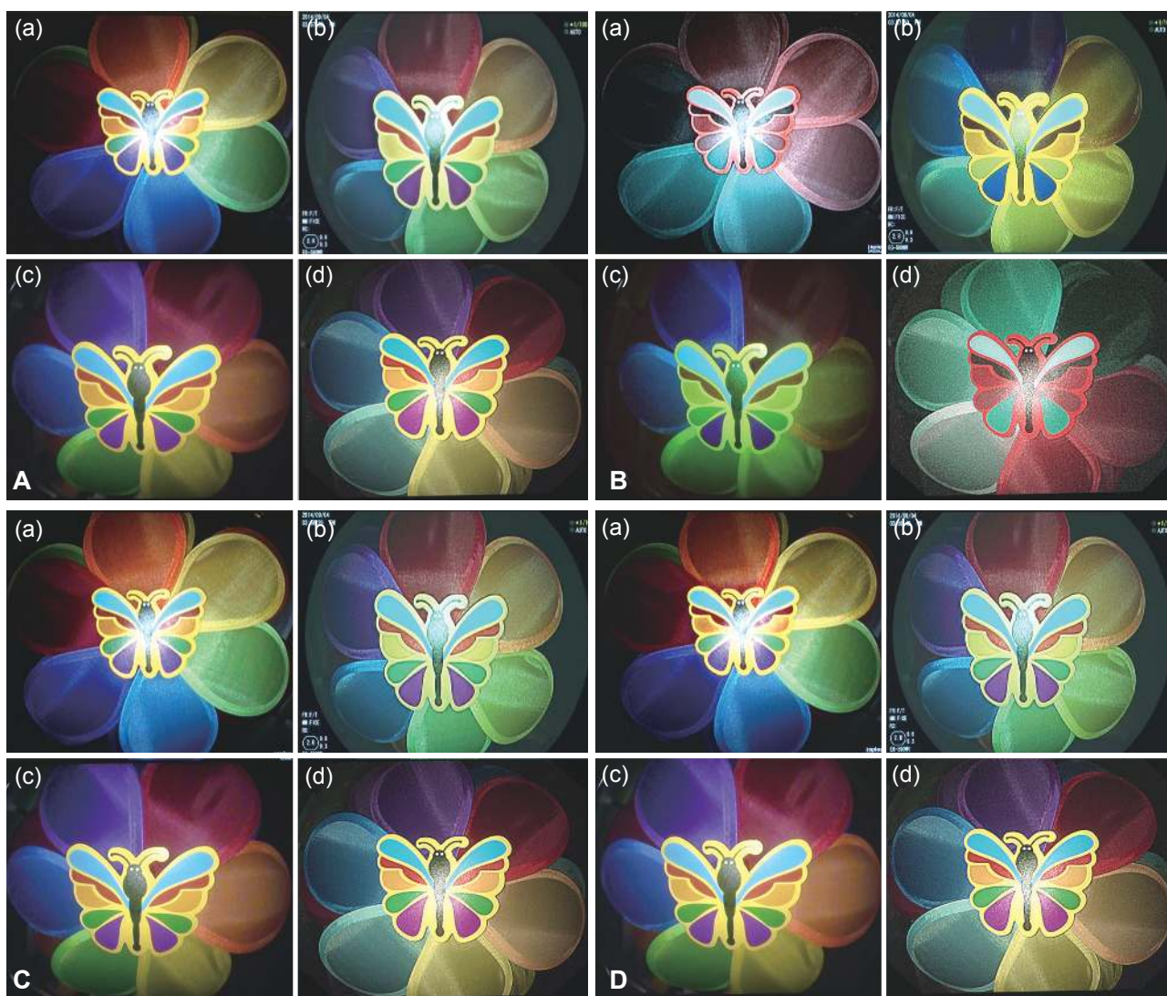
Fig. 1. Butterfly pattern ( in vitro ) taken according to each endoscopy company, analyzed on each point of evaluation, namely (A) definition, (B) boundary, (C) brightness, and (D) light and shade.
