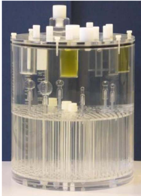
Fig. 1 Esser PET phantom with additional coplanar hot spheres of 4, 5, 6, 8, 12, and 20 mm, attached to the bottom of the phantom
