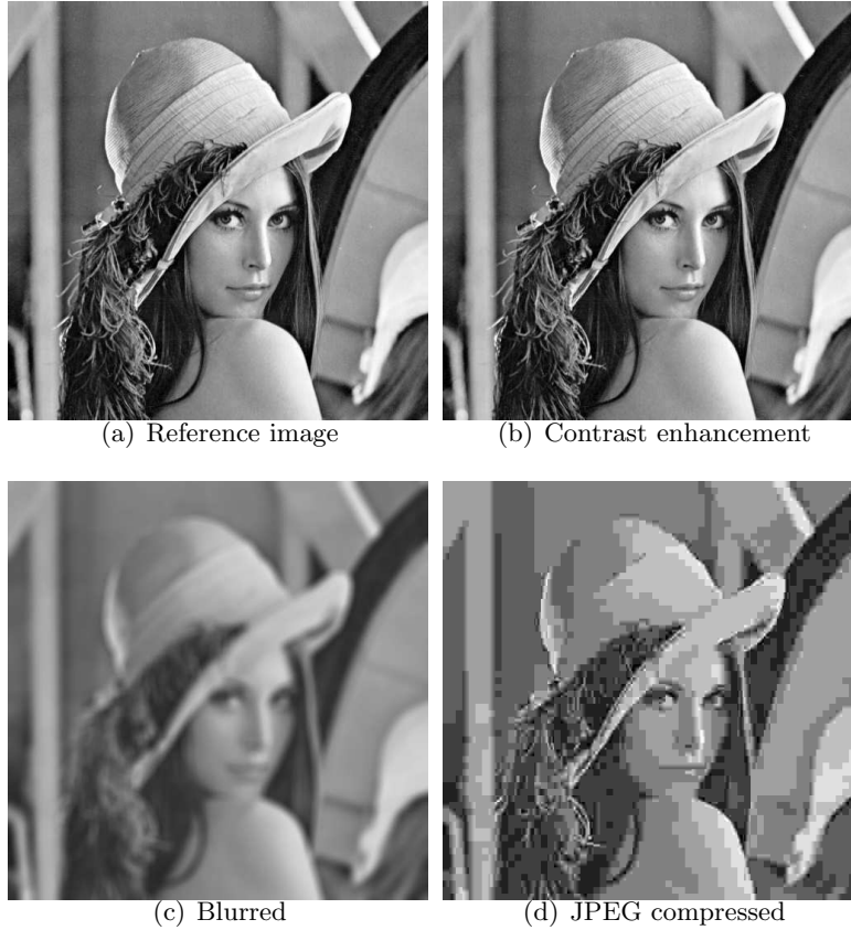
Figure 11: The VIF has an interesting feature: it can capture the effects of linear contrast enhancements on images, and quantify the improvement in visual quality. A VIF value greater than unity indicates this improvement, while a VIF value less than unity signifies a loss of visual quality. (a) Reference Lena image (VIF = 1.0). (b) Contrast stretched Lena image (VIF = 1.17). (c) Gaussian blur (VIF = 0.05) and (d) JPEG compressed (VIF = 0.05).
