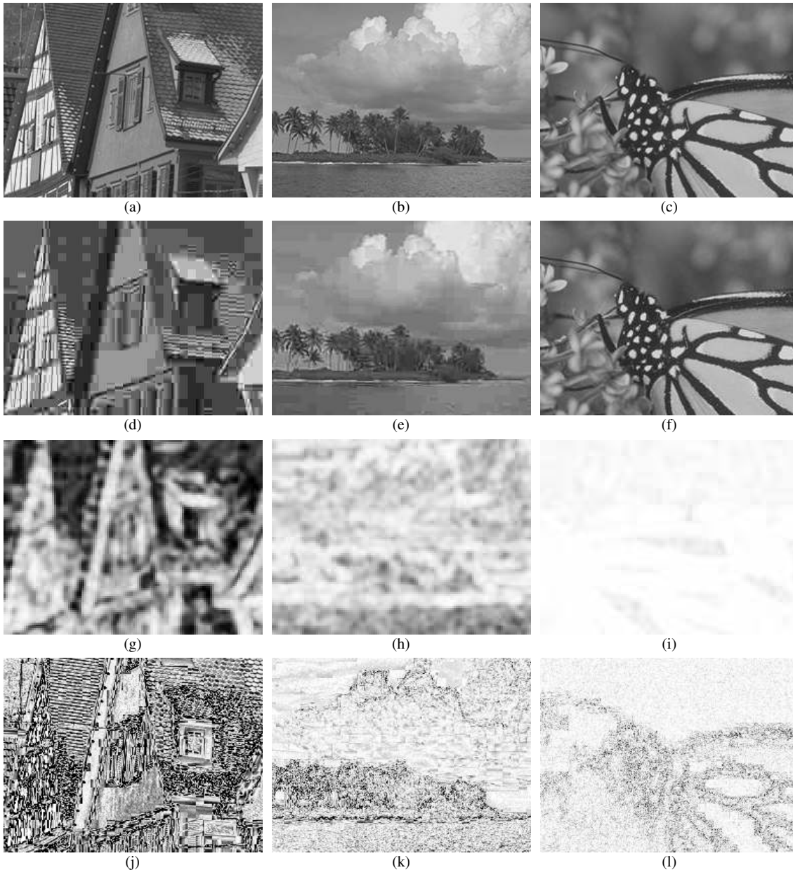
Fig. 6. Sample JPEG images compressed to different quality levels (original size: 768 \times 512 ; cropped to 256 \times 192 for visibility). (a), (b) and (c) are the original “Buildings”, “Ocean” and “Monarch” images, respectively. (d) Compressed to 0.2673 bits/pixel, PSNR = 21.98dB, MSSIM = 0.7118; (e) Compressed to 0.2980 bits/pixel, PSNR = 30.87dB, MSSIM = 0.8886; (f) Compressed to 0.7755 bits/pixel, PSNR = 36.78dB, MSSIM = 0.9898. (g), (h) and (i) show SSIM maps of the compressed images, where brightness indicates the magnitude of the local SSIM index (squared for visibility). (j), (k) and (l) show absolute error maps of the compressed images (contrast-inverted for easier comparison to the SSIM maps).
