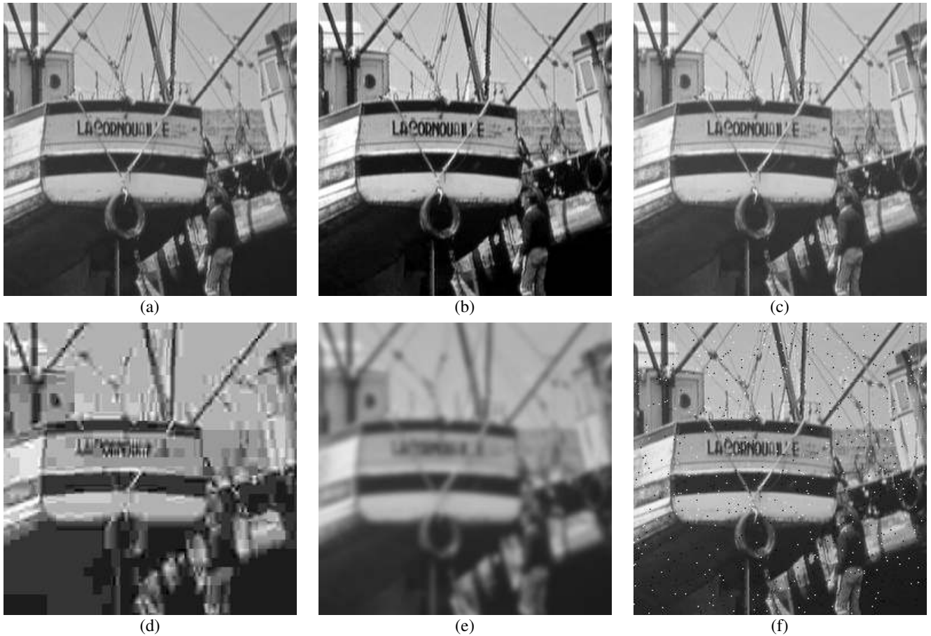
Fig. 2. Comparison of “Boat” images with different types of distortions, all with MSE = 210 . (a) Original image (8bits/pixel; cropped from 512 \times 512 to 256 \times 256 for visibility); (b) Contrast stretched image, MSSIM = 0.9168 ; (c) Mean-shifted image, MSSIM = 0.9900 ; (d) JPEG compressed image, MSSIM = 0.6949 ; (e) Blurred image, MSSIM = 0.7052 ; (f) Salt-pepper impulsive noise contaminated image, MSSIM = 0.7748 .
