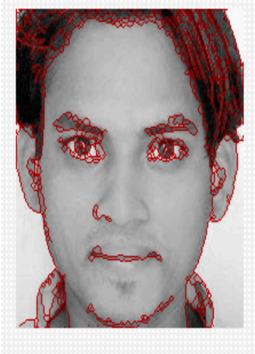
Fig 1: Template extraction of the highlighted features of the image.
