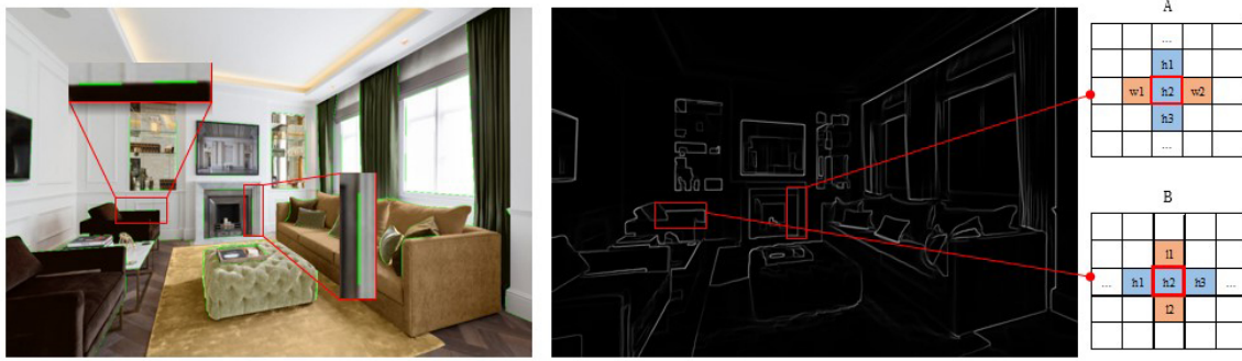
Figure 7: Example of holes (left); Scene edge detection (middle); Hole judgment diagrams (right), for vertical (A) and horizontal (B) holes, respectively.
