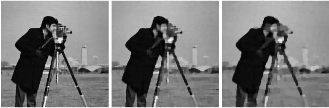
Figure 6. Reconstruction results from (20), where f contains impulsive noise corrupted partial average convolution data (5% entries of PK\bar{u} are corrupted randomly by either \min(PK\bar{u}) or \max(PK\bar{u}) , each at probability 0.5). \mu = 10^2 in (20) and \epsilon = 10^{-3} in (16). From left to right: sample ratios are 30%, 10% and 5%, (SNR, CPU, Iter) = (14.0dB, 9s, 86), (11.5dB, 9s, 92), and (10.2dB, 10s, 104), respectively.
