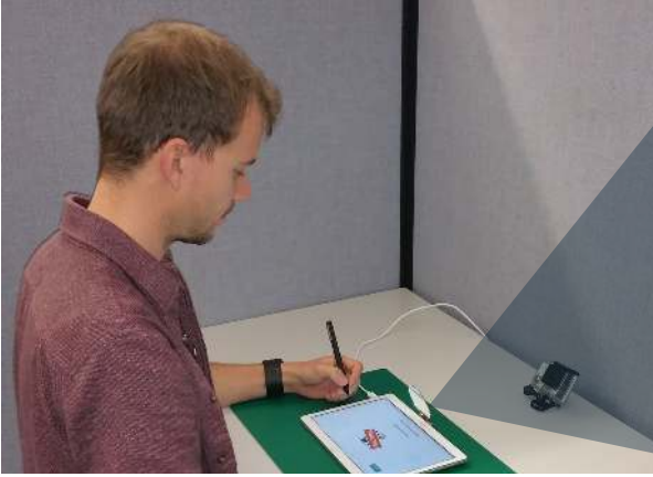
Figure 1: The hardware setup. A user is working on the tablet (a). A mirror is attached to the tablet using a hinge (b). Due to the mirror reflections, the field of view of the front camera is changed so that the face of the participant is visible (c).
