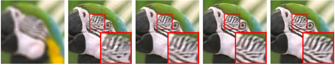
Fig. 5. Image deblurring performance comparison on Parrots image ( 9 \times 9 uniform blur, \sigma_n=2 ). From left to right: blurred and noisy; FISTA [40] (PSNR=28.88 dB); BM3D [41] (PSNR=29.74 dB); ASDS-Reg [15] (PSNR=30.17 dB); Algorithm 2 (PSNR=30.70 dB).
