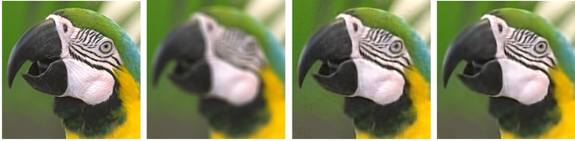
Fig. 3. The deblurred Parrot image by the proposed methods ( 9 \times 9 uniform blur with \sigma_n = \sqrt{2} ). From left to right: original image; blurred and noisy; deblurred by Algorithm 1 ; deblurred by Algorithm 2 .
