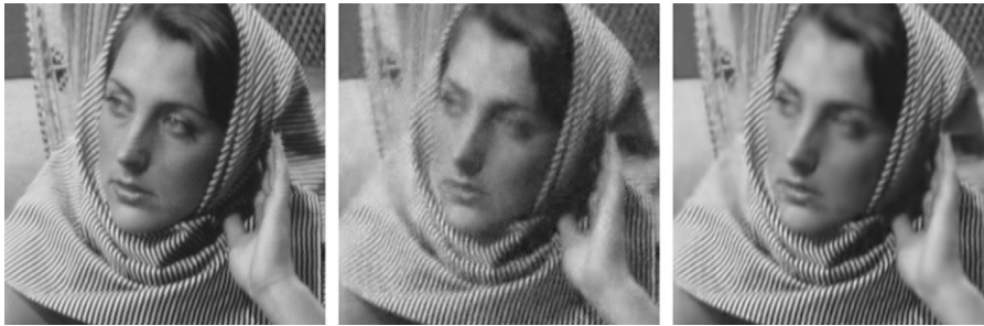
Fig. 11. The reconstructed Barbara images by the proposed methods (using M=0.2N measurements). From left to right: Original image; reconstructed image by Algorithm 1 ; reconstructed image by Algorithm 2 .
