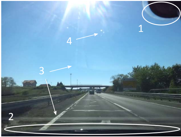
Fig. 1: A typical traffic scene. Note the camera mount (1), the dashboard (2), reflections of car interior (3) and a speck of dirt (4)
