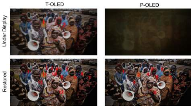
Figure 8: Face detection performance before and after applying restoration. Without display, the original face recall rate is 60%. Covering the camera with T-OLED or P-OLED will decrease the recall rate to 8% and 0%. After image restoration, the recall rates recovered back to 56% and 39%.
