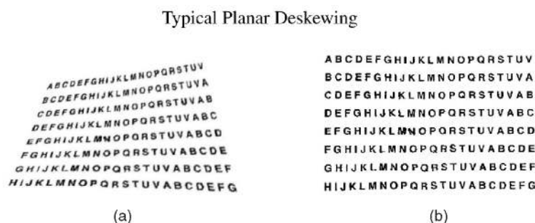
Fig. 3. An example of typical planar deskewing algorithms. (a) An image with content that is not raster aligned. (b) A homography is used to align the content with the raster image.
