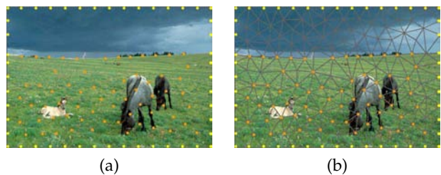
Fig. 2. Mesh generation. (a) Input image with boundary (the yellow dots) and feature points (orange ones) evenly distributed. (b) Delaunay triangulation result. The rest mesh points are added automatically with a distance threshold to maintain mesh uniformity.
