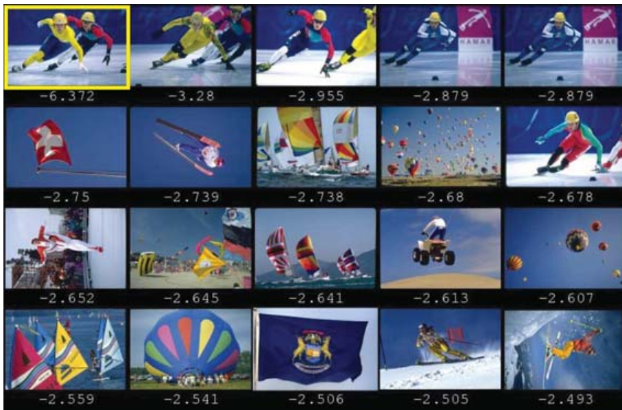
Fig. 5. Sample query results for a combined search using z-transform. Below each image, the average of the z-values of the chromaticity, the luminance, and the Fourier histogram distances is shown. The query image is shown at the top left.
