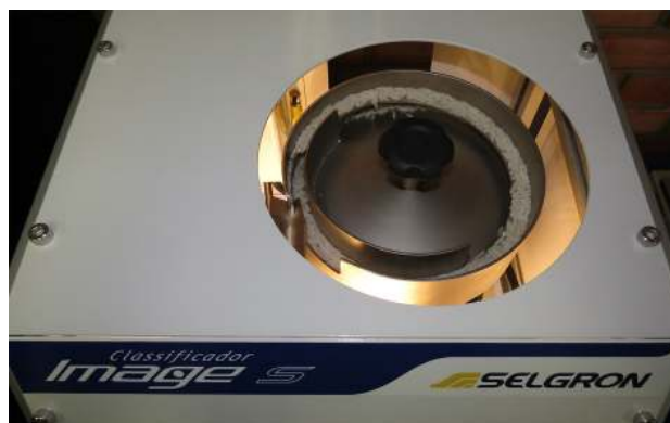
Figure 2. Image running a milled rice sample at the helical vibratory plate.
