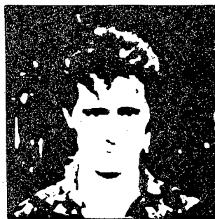
(c) energy threshold = 25, 15 quant. levels, # segments = 697
