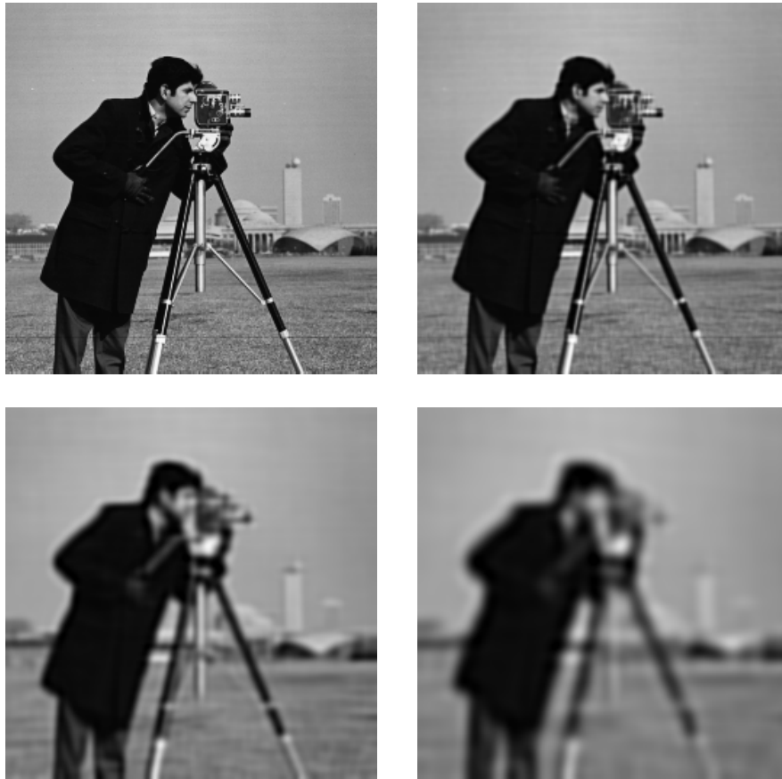
Fig. 7. Hyper-diffusion processing of the cameraman image, given at normalized times 0 (top-left), 0.1 (top-right), 1 (bottom-left), 10.
