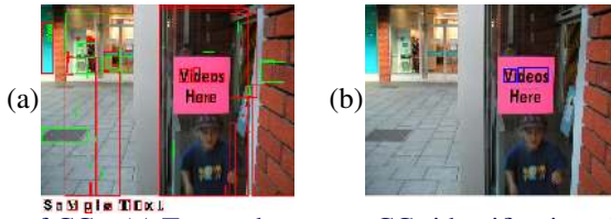
Figure 6: Clustering of CCs. (a) Text and non-text CCs identification. (b) Merging text CCs to generate the final result.
