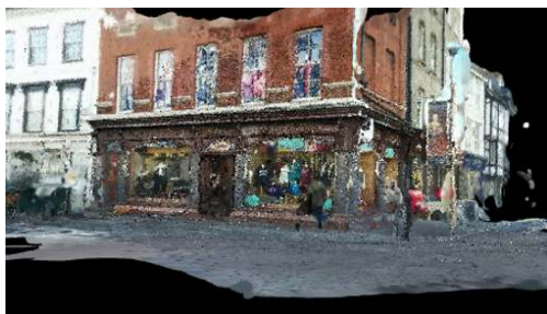
Figure 4. Example of a rendered image from the 3D model. The 3D model is generated from the captured training images.
