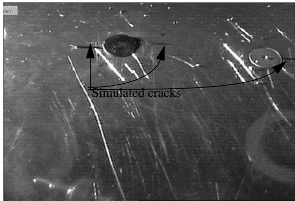
Fig 10a. Metal surface with three synthetic cracks and other crack like features
