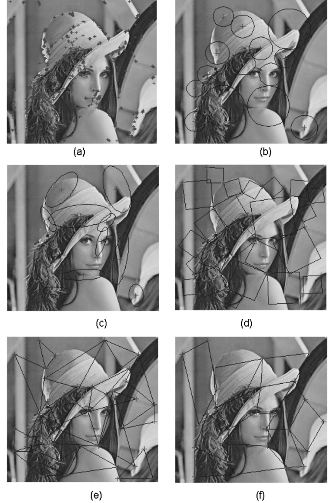
Fig. 4. (a) Scale-space Harris points. Finally selected invariant regions for watermarking using (b) characteristic scale, (c) shape adaptation of the Gaussian kernel, (d) feature-point set with Q = 2 , (e) feature-point set with Q = 3 , (f) feature-point set with Q = 4 . The radius of the circles in (b) is eight times the characteristic scale of the Harris point. The major and minor axes of the ellipses in (c) are 11 times that of the original value.
