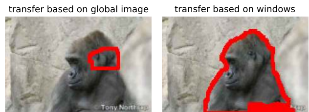
Fig. 3 An example to demonstrate the advantage of window-level segmentation transfer over global transfer. In both cases the transferred mask M is used to guide a GrabCut-like segmentation process of Sect. 4.1. The two methods differ in how M is obtained
