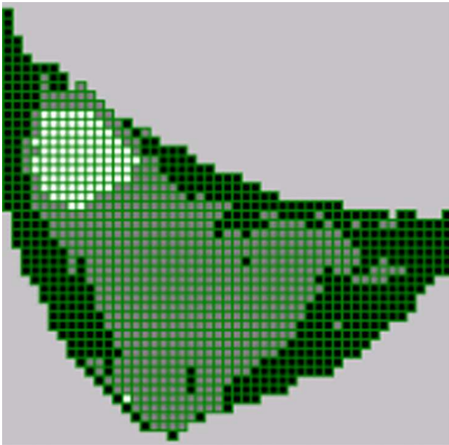
Figure 5 The FEM Mesh of the Breast. The selected region is meshed by cuboidal elements. The color of black denotes fat; gray parenchyma; and white tumor. The green lines are the boundary of elements. Though only one slice is shown here, elements are also generated for some other slices so that the 3D FEM mesh of the Breast is obtained.
