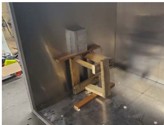
FIGURE 10. Photograph of the rectangular aluminum block on the internal face of the container.
