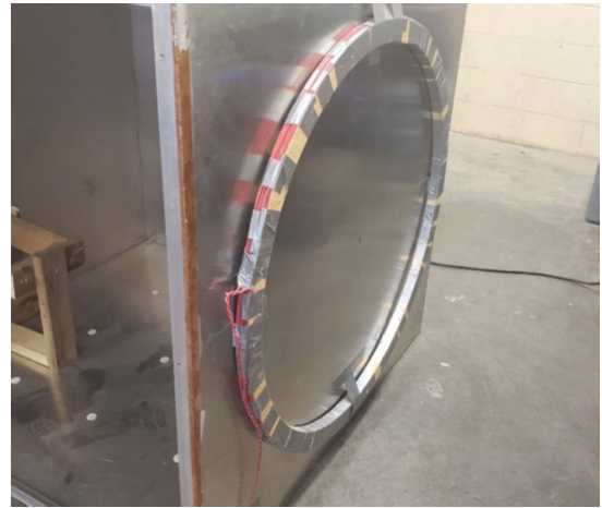
FIGURE 9. Photograph of the transmitting loop source fastened to the external face of the container.
