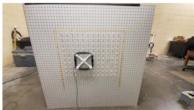
FIGURE 11. Photograph of the receiver array to scan for the hidden aluminum object.
