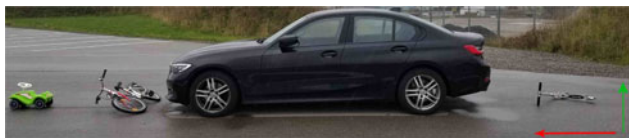
Fig. 12. The first measurement scenario. Red arrow indicates the driving direction and the green arrow shows the direction of the SAR sensor bore-sight.
