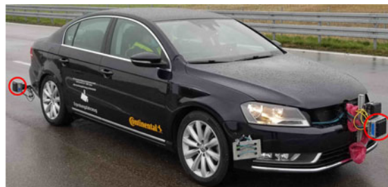
Fig. 1. Measurement set-up for SAR. Height of rear-right sensor: 40 cm, height of front sensor: 50 cm.
