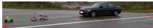
Fig. 14. Repeat of scenario from Fig. 12 with greater spacing between the objects. Red arrow indicates the driving direction and the green arrow shows the direction of the SAR sensor bore-sight. The scooter is encircled in red in the background.
