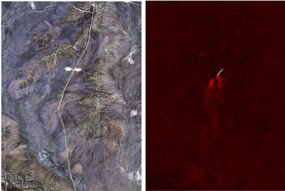
Fig. 8 (Left) True color segment of an AVIRIS-NG flight line acquired in 2014 from the Four Corners Campaign with spectroscopic data available from http://avirisng.jpl.nasa.gov . (Right) A \text{CH}_4 retrieval using the technique of Thompson et al. (2015b) shows a plume emanating from a gas well pad. Brighter pixels correspond to higher local enhancements
