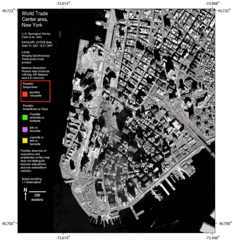
Fig. 6 Serpentine and amphibole minerals map of the lower Manhattan area, New York City, New York, USA. Image sourced from Clark et al. (2006)
