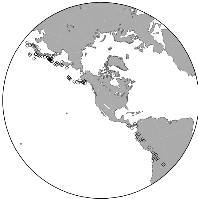
Figure 2. Global distribution of the 84 earthquakes (diamonds) with m_b \geq 5.6 , used for calculating the 2706 receiver functions used in this study. The events are teleseisms from epicentral distances of 35\text{--}95^\circ , with great circle paths that are \pm 10^\circ of the mean array azimuth. The RISTRA seismometer deployment (Figure 1) is depicted as great circle swath.
