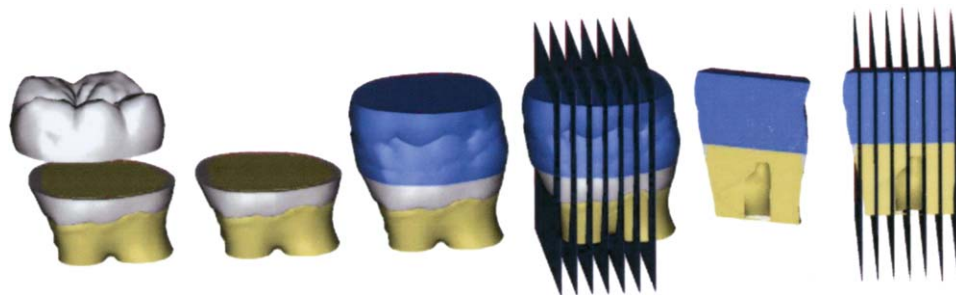
Fig. 2. Schematic representation of preparation of composite resin-dentin beams in “nontrimming” version of microtensile bond test.
