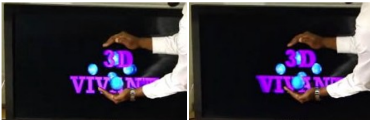
Figure 5: Two perspective views of a 3D holoscopic image on a commercial 3D autostereoscopic display. Parts of the 3D holoscopic image on the screen (such as the 1 st Globe) can be seen to be at the same depth as the image of the hand.
