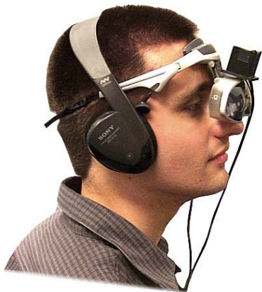
Fig. 4 - A user wearing a head-mounted display with an orientation tracker.
