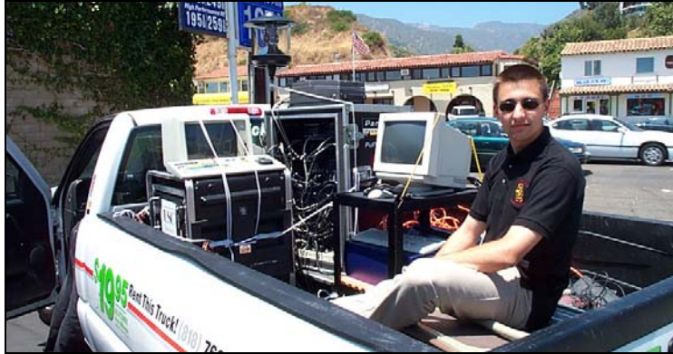
Fig. 9 – A mobile panoramic video recording setup.
