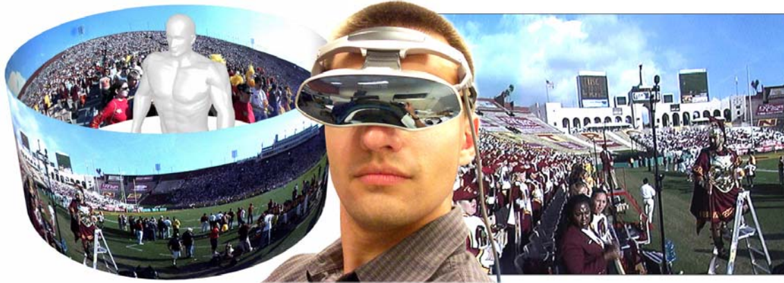
A user navigates a panoramic video environment using a head-mounted display and tracker.
