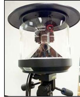
Fig 1 - Our five sensor panoramic camera system.
