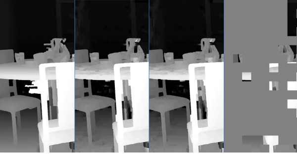
Fig. 3: Example for different depth signals in the H-DSDE system. From left to right: source depth ( D ), DSDE depth ( D^+ ), hybrid depth ( D_H^{*+} ), decoded partial depth ( D_{part}^* ).
