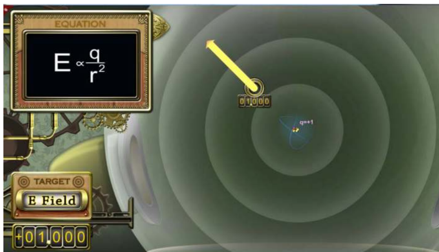
FIGURE 3 | Screen capture of a later trial. The vector is longer and the dynamic equation for the electric field has changed as well. Note that E is much larger and the r is smaller (compared to Figure 2 ), these components change dynamically as the hand moves in real time.
