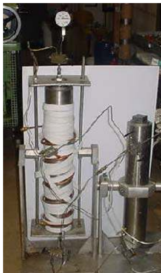
Figure 10: Fluid Transfer Vessel (C)
