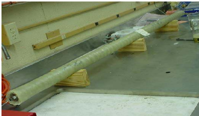
Figure 8: 6-ft Berea Core with Epoxy Coating (B)
