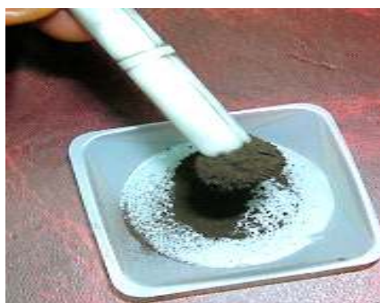
Figure 1. Magnetic performance of the fabricated magnetic amine-functionalized silica gel nano-hybrid material (MANSG).
