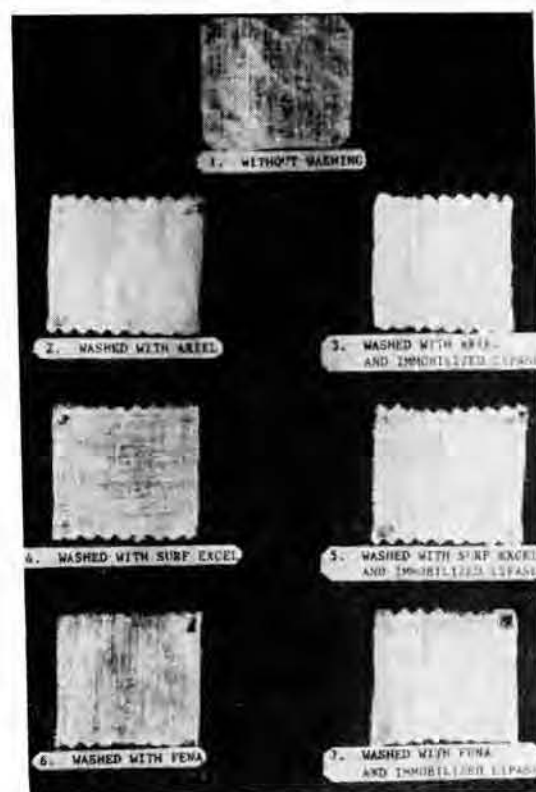
Fig. 4—Washings of cotton cloth having mustard oil stains in detergent with and without immobilized lipase.
