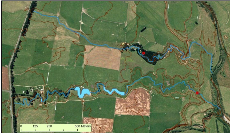
Figure 4.17: Location of knickpoints (red circles) in the unregulated and regulated catchments. Contour lines are plotted at 5 m intervals.
