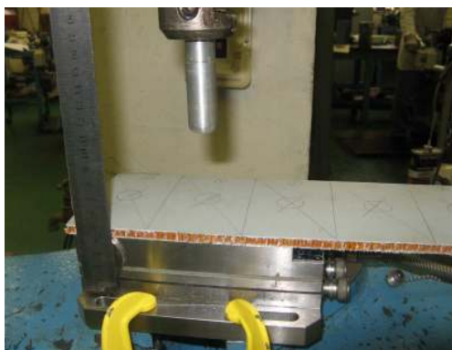
Figure 4. Left, setup used to create the impact damage on the specimen with typical core damage obtained as depicted in the image to the right.
