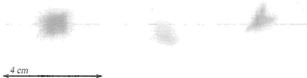
Fig. 20. Impact point of 5 J impacted specimens ( 10 \times 10 cm), backlight picture.
