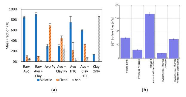
**Figure 4.** Characterization of raw materials, biochars, and hydrochars (error bars indicate one standard deviation) including (**a**) proximate analysis results (clay-free basis) and (**b**) surface area.
