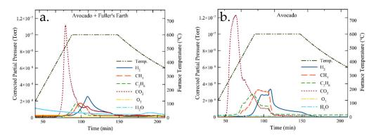
Figure 2. Gas emissions from pyrolysis of (a) avocado pits with 20% bentonite clay and (b) avocado pits.
