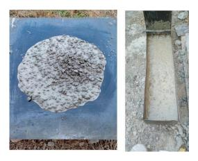
Figure 3. Slump test (left) and L-box test (right).
