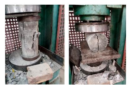
Figure 7. Compressive strength testing (left) and split tensile strength testing (right).
